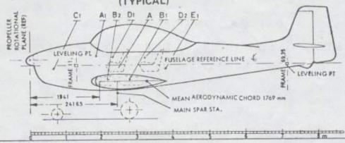
C. G. LOCATION IS REFERENCED TO PROPELLER ROTATIONAL PLANE
