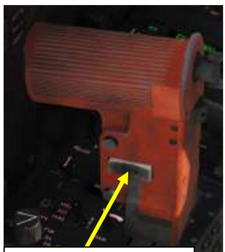
Radio Selection Switch (selects either COM1 or COM2 radio)
