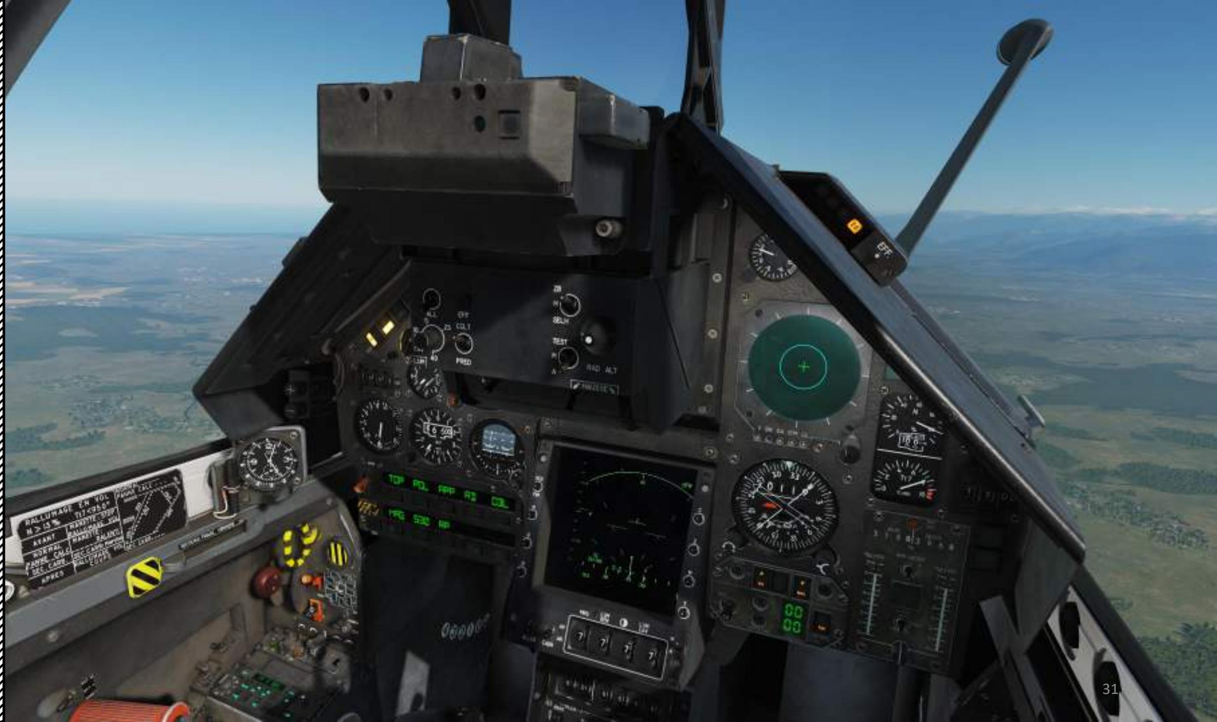
VTB Radar Control Panel: Radar Visualisation Tête Basse
