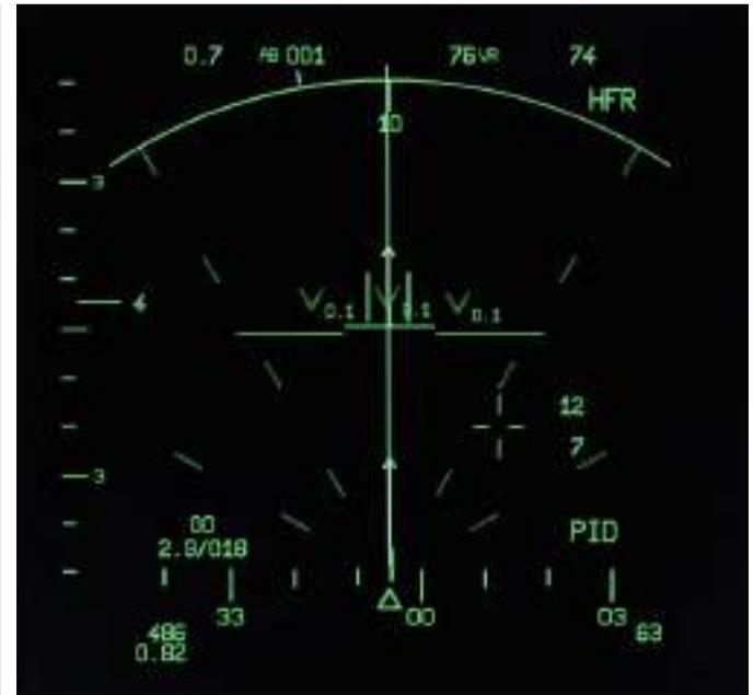
RADAR IN TWS (Track While Scan)/PID MODE
