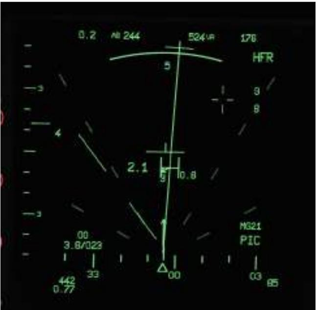
RADAR IN STT (Single Target Track)/PIC MODE
