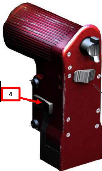
Radio Selection Switch (selects either COM1 or COM2 radio)
