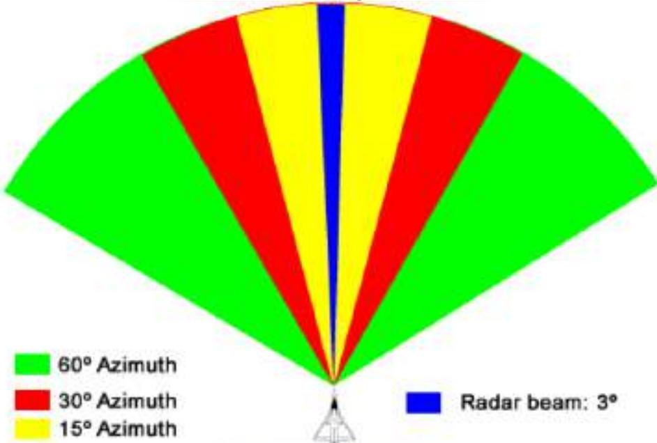
Figure 22 Horizontal Radar aperture
