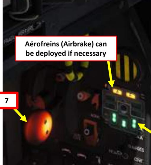
Green Light = Landing Gear Deployed
