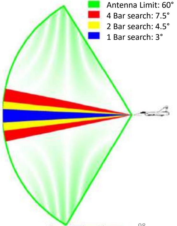
Figure 23 RDI radar vertical coverage
