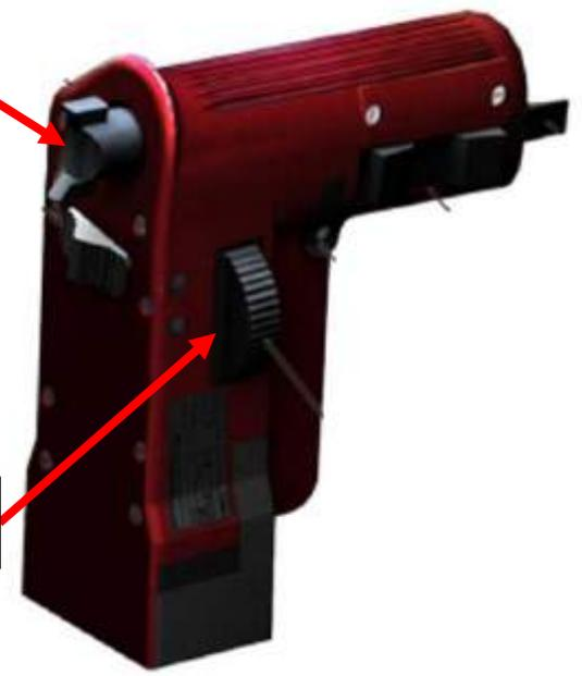
Antenna Elevation Thumbwheel
