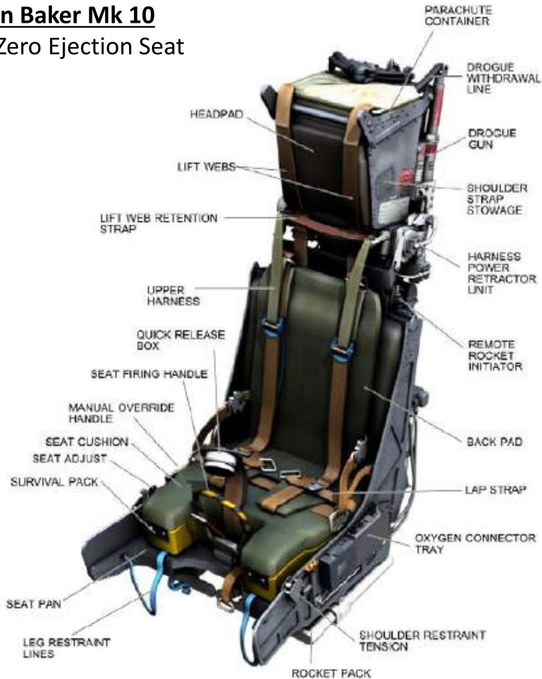
A **zero-zero ejection seat** is designed to safely extract upward and land its occupant from a grounded stationary position (i.e., **zero** altitude and **zero** airspeed), specifically from aircraft cockpits. The zero-zero capability was developed to help aircrews escape upward from unrecoverable emergencies during low-altitude and/or low-speed flight, as well as ground mishaps. Before this capability, ejections could only be performed above minimum altitudes and airspeeds.
