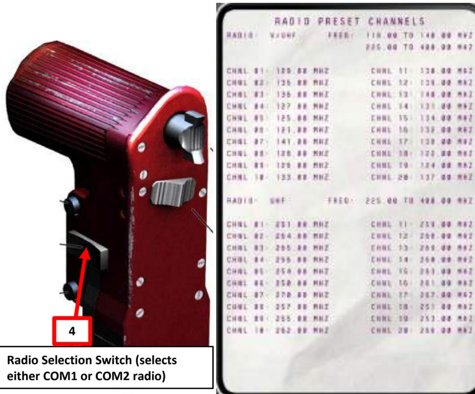
Radio Selection Switch (selects either COM1 or COM2 radio)
