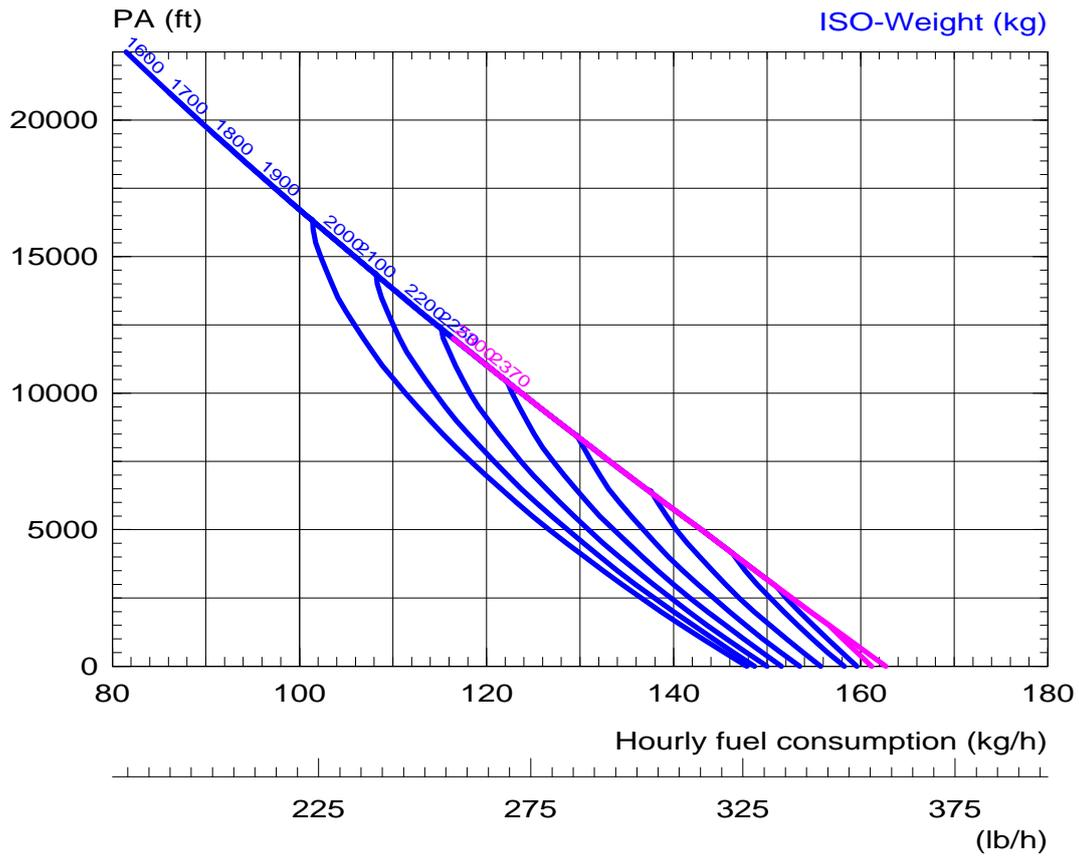
Note : Typical consumption with clean baseline aircraft and new engine.
