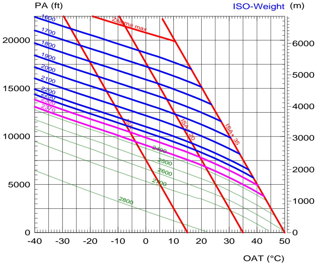
Note : ISO weight curves from 2,300 to 2,800 kg are curves with external load.
