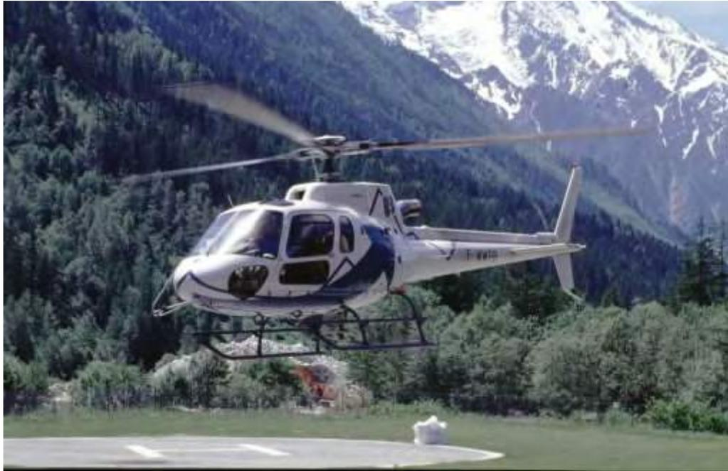
The AS350 B3 is "the high performance" version of the single engine ECUREUIL range, beating every other single engine helicopter in its category. It fulfils the FAR 27 regulation for VFR operation by day and night <sup>1</sup>. It offers a Maximum Internal Gross Weight of 2,370 kg / 5,225 lb <sup>2</sup> and a Maximum all-up weight of 2,800 kg / 6,172 lb in external load configuration. This makes the helicopter perfectly suited for:
